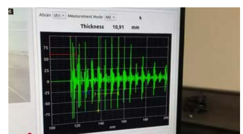
Live thickness measurements with A-scans and tuning options
