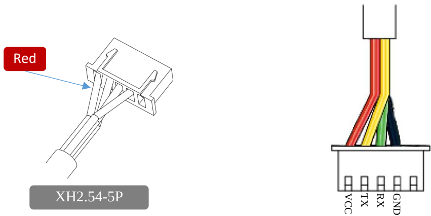
Figure 2-5 RPLIDAR Power Interface Definition
