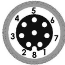
Figure 7.2 – M8 port pin locations
