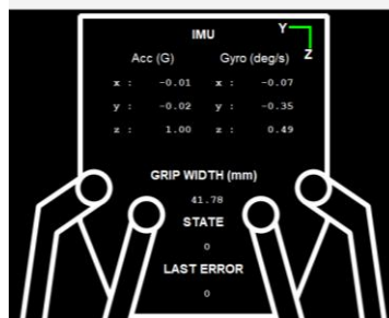
Figure 11.6 – Visualisation Software: Visualisation of IMU data, State and Last Error
