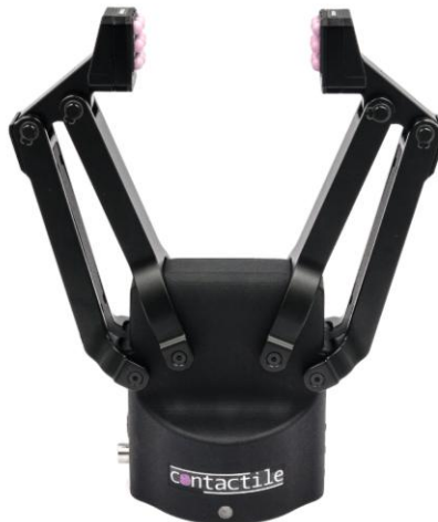
Figure 3.1 – The GAL2 2-Finger Angular Lead-Screw Gripper (Beta v1.1) with integrated PapillArray Tactile Sensors.
