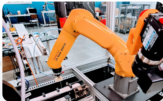
Robotic box feeding and erecting
