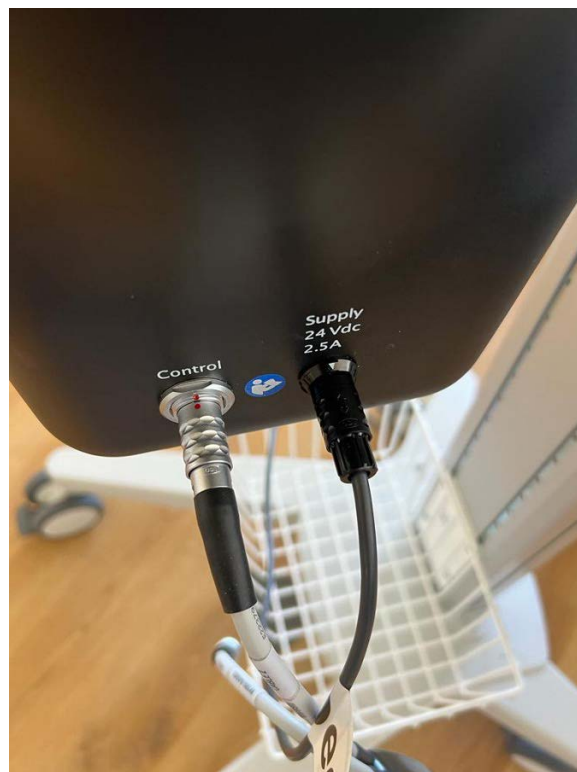
Figure 39: Example of a Data Cable correctly connected
