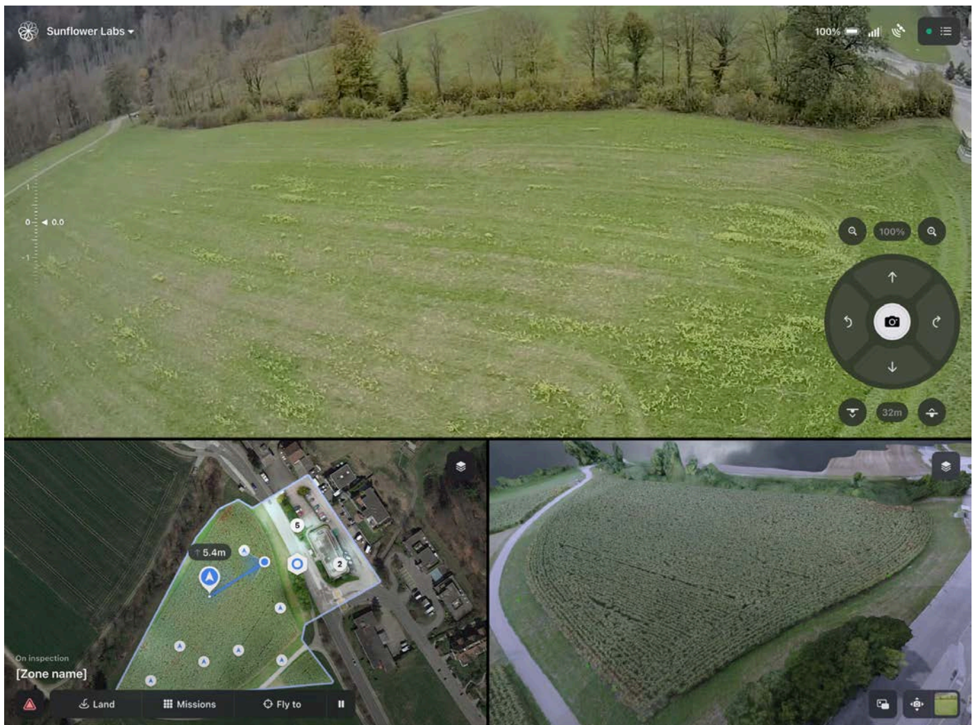
Figure 7-3 - Control Station (CS) application in split view
