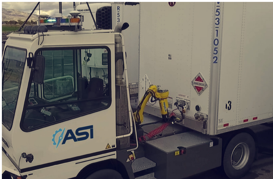
ASI equipped autonomous yard truck connects to trailers, uses a robotic arm to connect air lines, then moves the trailer to a dock door or other parking stall (2022).
