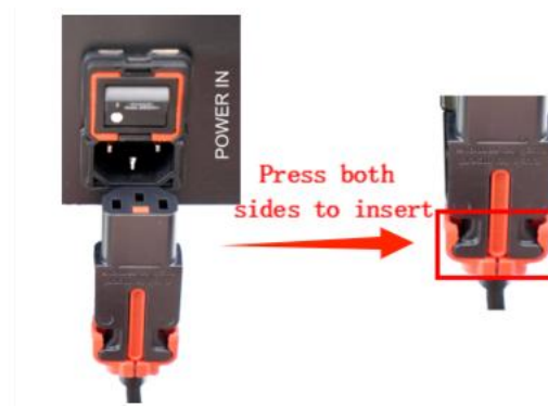
Figure 73 Diagram of mains power connection
