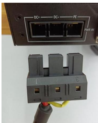
Figure 76 Diagram of power box cable connection
