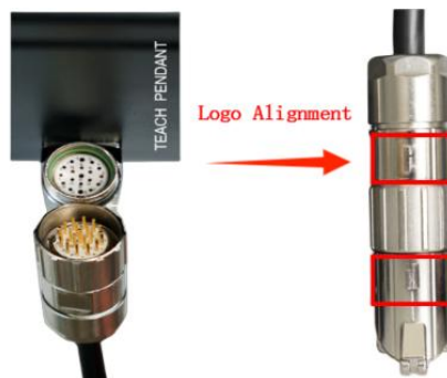
Figure 71: Cable connection diagram of the teaching device
