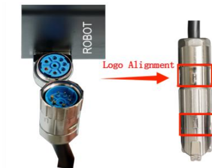
Figure 72 Diagram of the robotic arm cable connection
