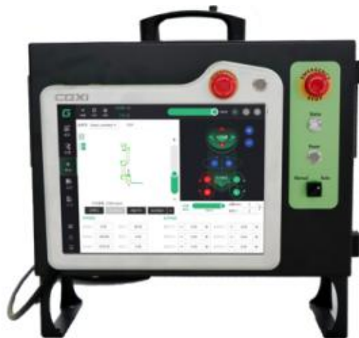
Figure 70 A physical picture of a teaching device hanging on a control cabinet hanger
