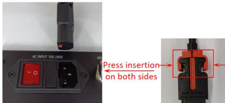
Figure 77 Diagram of mains power connection
