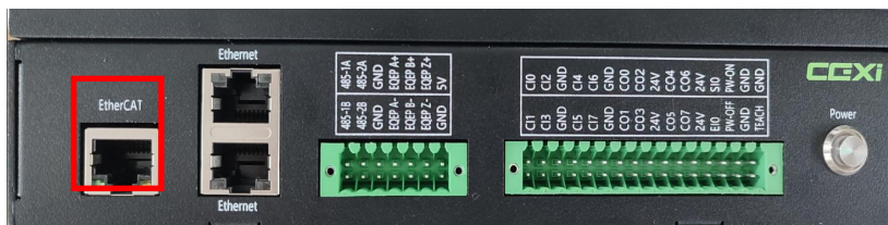
Figure 115 Controller extends EtherCAT interface
