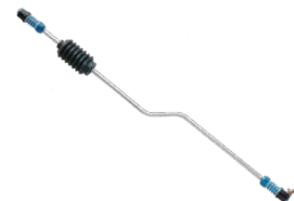
Steering Arm Assembly HEPSTAA1000
