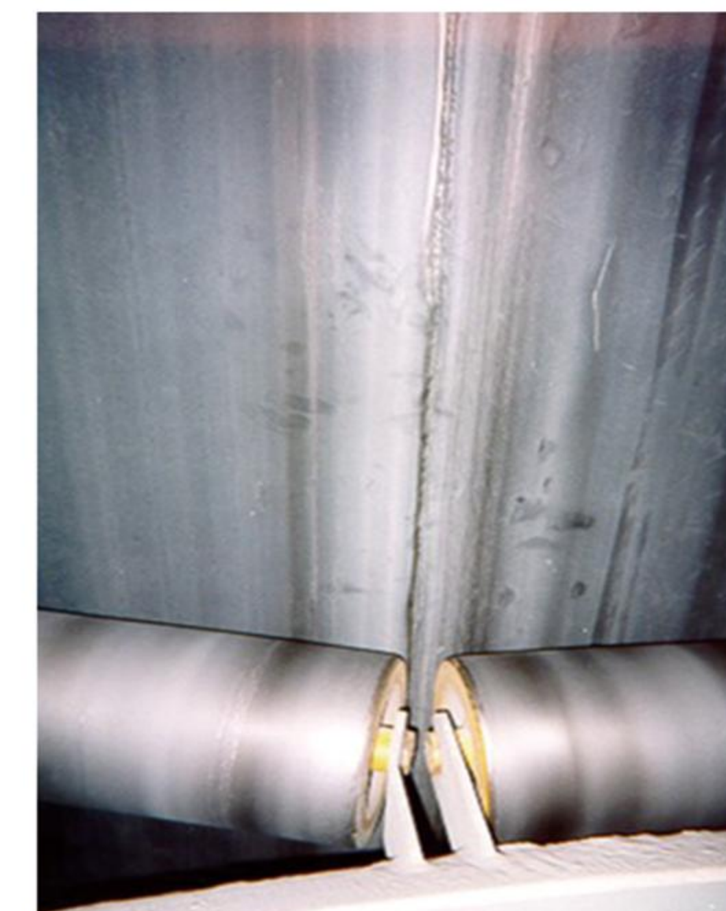
The idler connection cover is faulty
