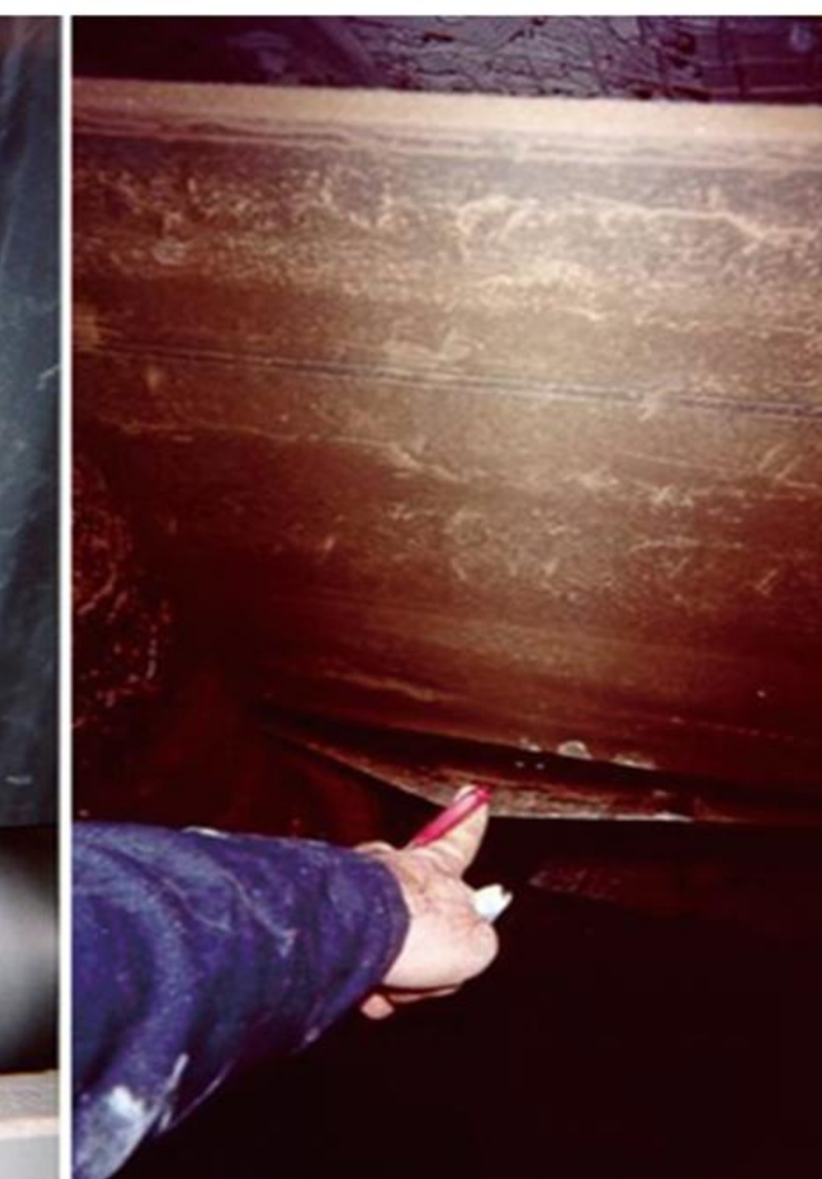
The idler connection cover is faulty
