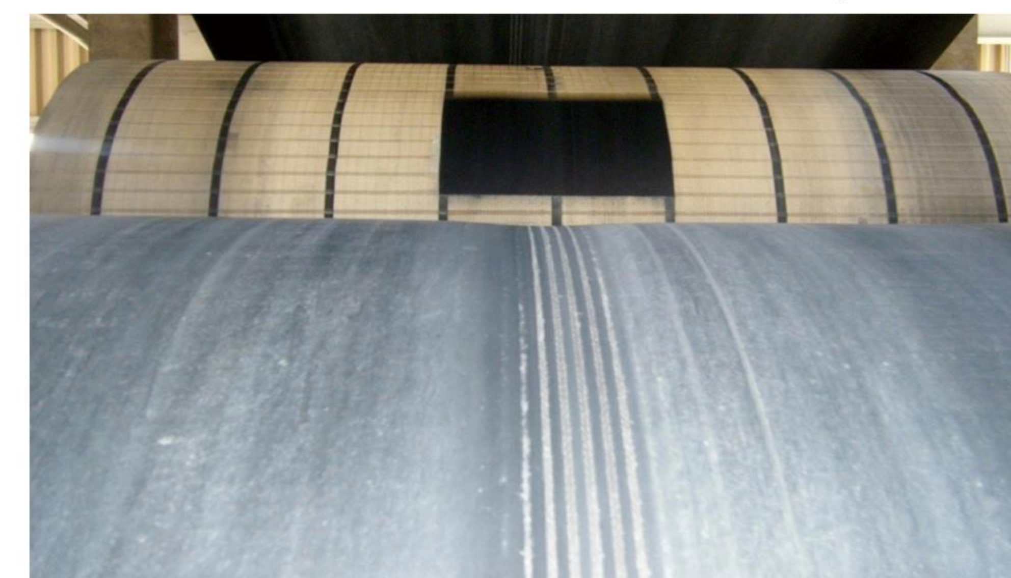
Bottom cover wear caused by ceramic cladding
